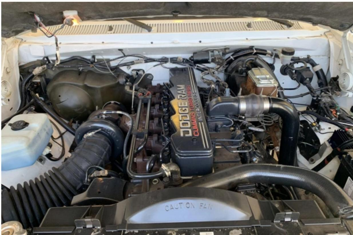
The 5.9-liter Cummins 6BT turbodiesel inline-six was factory-rated at 160 horsepower and 400 lb-ft of torque when new and features an intercooler. The valve cover gasket and coolant are said to have been replaced in 2020, and an oil change was also performed.
