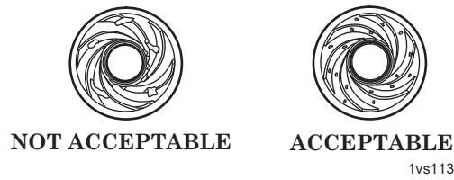
Figure 13. Bore Inspection.
