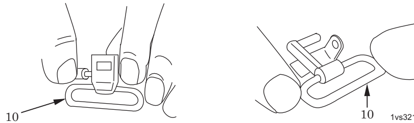
Figure 10. Attaching Swivel to Lanyard.
