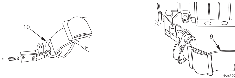
Figure 11. Securing Swivel and Lanyard.
